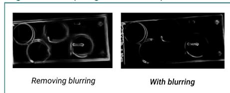
Deblurring improves HED algorithm for detecting coverslips
