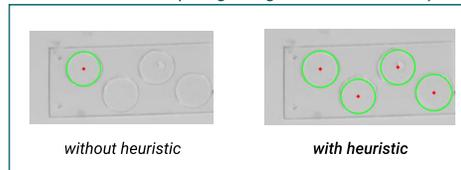
Adding the heuristic, based on standard microscopy slide dimensions, increasing location prediction significantly using CHT algorithm
